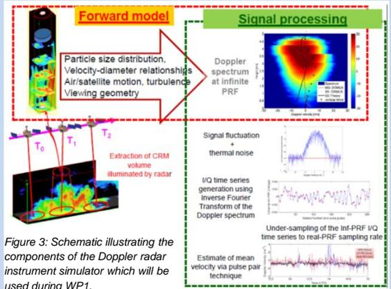
Figure 3: Schematic illustrating the components of the Doppler radar instrument simulator which will be used during WP1.
