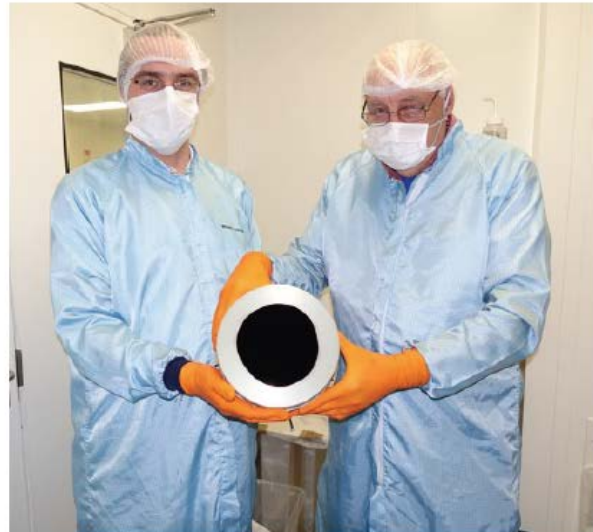
Breadboard blackbody cavity with carbon nano-black coating developed in a previous UKSA project
