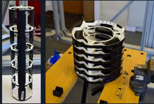
Secondary reflector deployment tower
