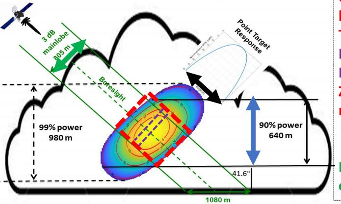
"frequency modulated pulse could potentially Improve range resolution" "RAIN-CUBE" 94GHz. Launch 2018. Vertical incidence. Pulse compression has > -80dB range sidelobes. **Canadian colleagues (Wolde & Nguyen)** have WIVERN pulse compression design. Try it out in phase zero on their aircraft. **Potential 100m range resolution. Purple dotted line in figure** Z value every 75m in vertical, derive rain rate from 94GHz attenuation of Z ~ 1.6dB/km per mm/hr of rainfall.
