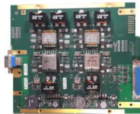
Central Power Distribution
