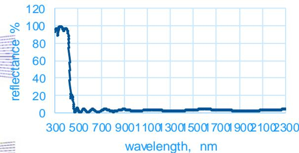
Sofradir wide spectral range CMT detector allows a 2 detector design also channel separation at ~ 420 nm reducing criticality of coregistration and Si detector design
