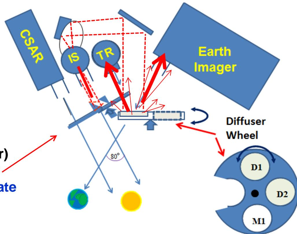
Note two diffusers for redundancy & reduced exposure/degradation. Mirror for higher illumination levels
