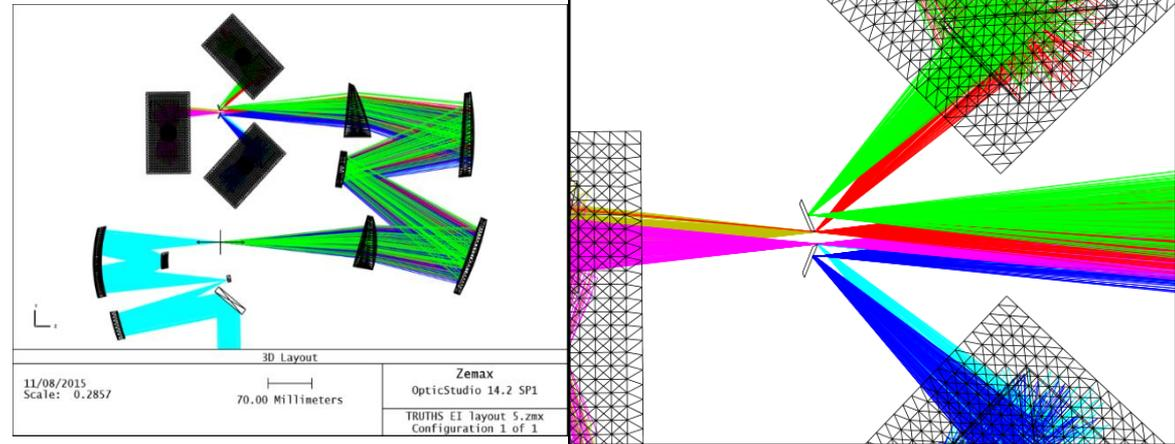
Original Baseline used single spectrometer but split to 3 detectors via a relay system – concern over detector number and knife edge mirrors for beam separation
