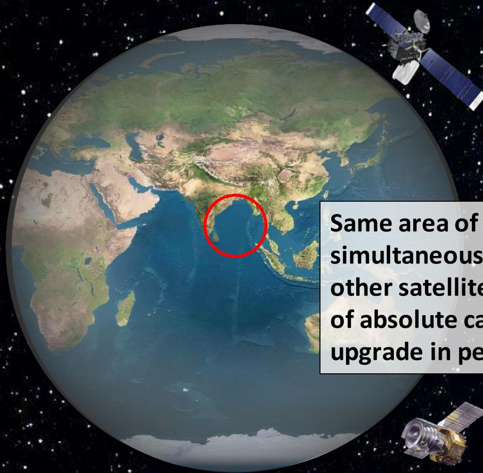
Same area of Earth viewed simultaneously by TRUTHS and other satellite enables transfer of absolute calibration and upgrade in performance
