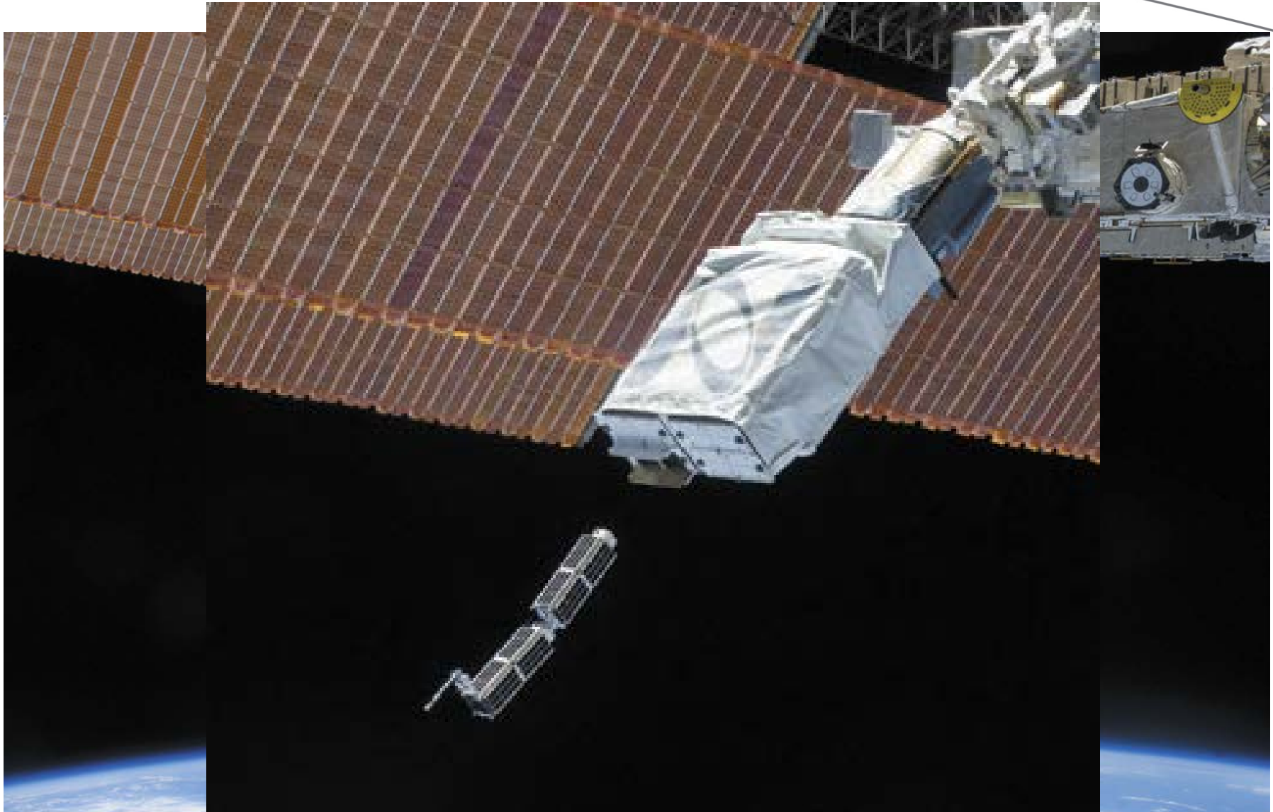
Two 30-centimetre CubeSats released from the ISS in February 2014
