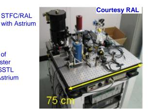
Laser heterodyne sounding in 4-150 µm range
