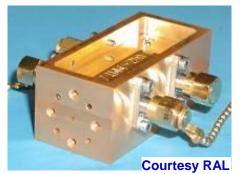
SHIRM 360 GHz image separator mixer using Schottky diode technology
