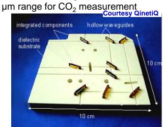
**Integrated Optics** Hollow Waveguide
