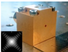
Quantum Cascade Laser (QCL) devices as a high-power source to pump heterodyne Schottky mixers
