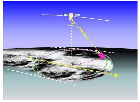
500km orbit **800km wide ground track**: Slant range 651km Conical scan 37.9° off-nadir (41.4° off zenith at surface)
