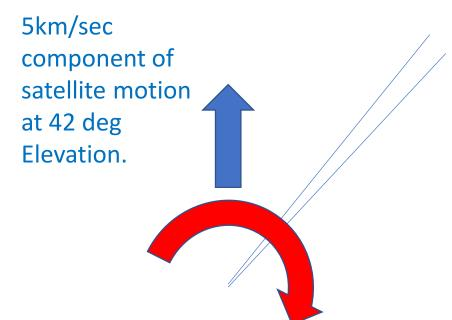
Radar beamwidth ~1 mrad (0.05degs) So induced wind shear up to 5m/s across the beam
