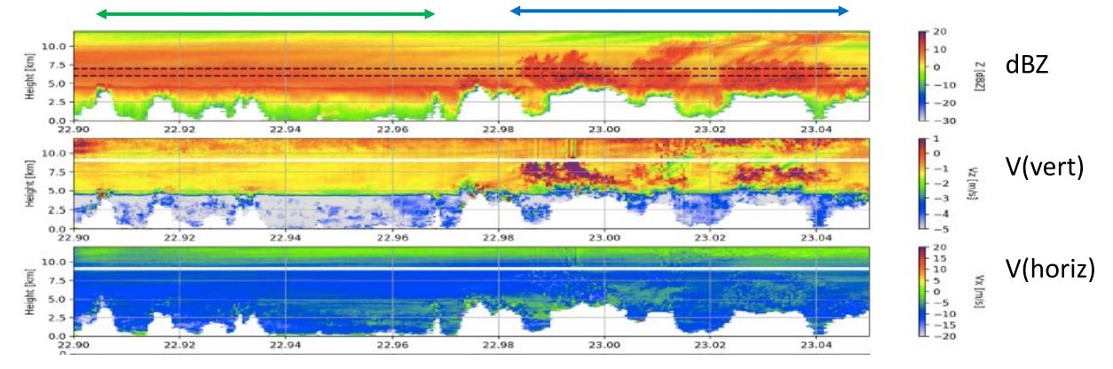
Can compute WIVERN line of sight (LOS) wind, and apparent HLOS = LOS (cos 41degs)<sup>13</sup>
