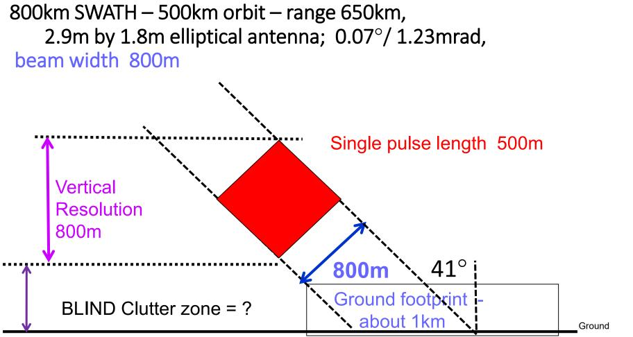
Canadian aircraft observation of 94GHz SURFACE CLUTTER AT 40deg incidence CLUTTER ZONE < ~1km over ocean, < ~ 2km over land.
