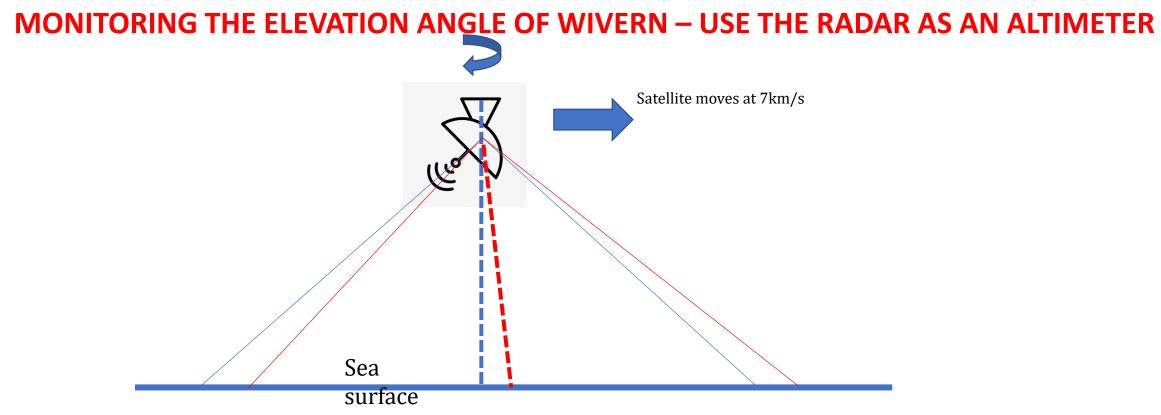
Blue – the range remains constant when the antenna rotates around an axis pointing to nadir. Red – the range varies sinusoidally if the radar rotates about an axis that is slightly off nadir.
