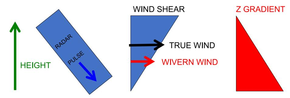
AEOLUS corrects for this effect using the known air density change with height. Ground-based operational C-band Doppler radars make same correction for vertical gradient of Z.
