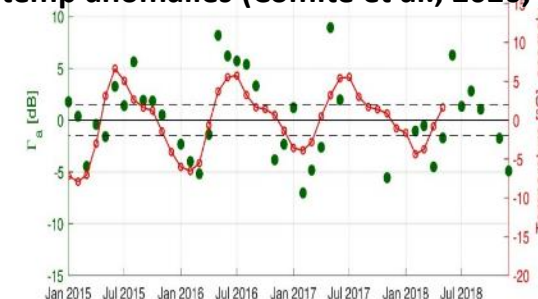
Siberian Permafrost, TDS-1 reflectivity (green) vs in-situ soil temp anomalies (Comite et al., 2020, in review)
