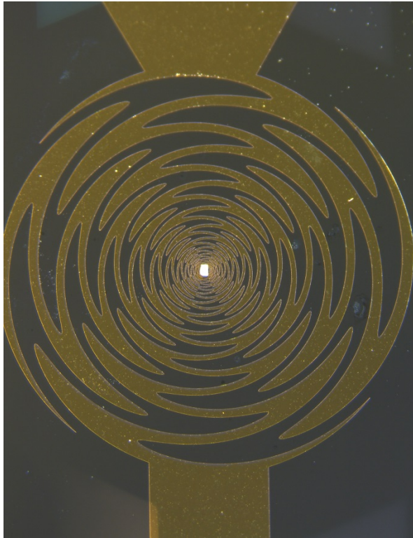
Broadband sinuous antenna with diode chip in centre
