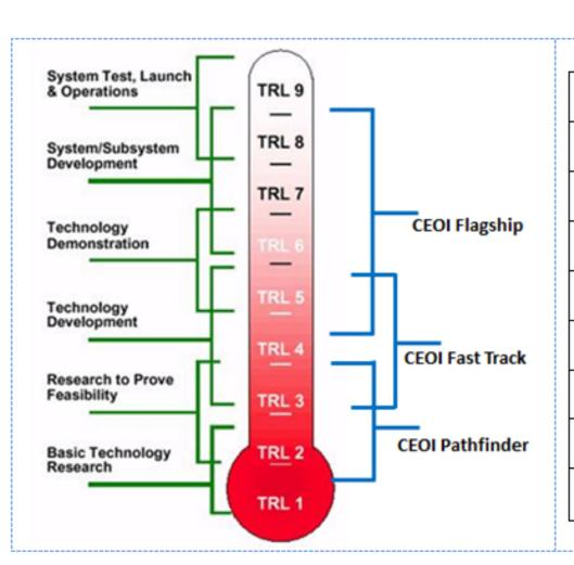
TRL9 - Actual system "flight proven" through successful mission operations
