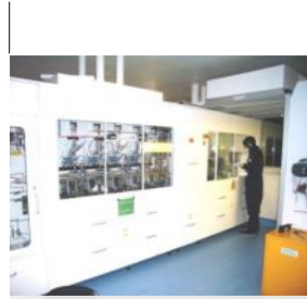
3 rd generation MCT growth on low cost 3" and 4" GaAs substrates
