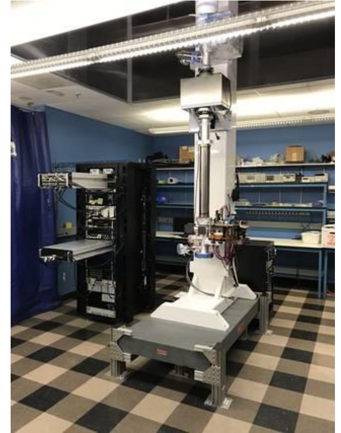
The Goddard-AOSense terrestrial proof-of-concept gravity gradiometer.
