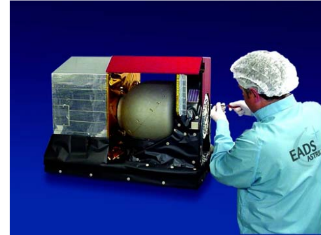
MHS - Microwave Humidity Sounder on Metop
