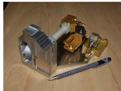
Example compact 0.5THz receiver
