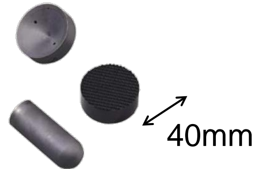
Fixed-Point Cells for Blackbody Sources
