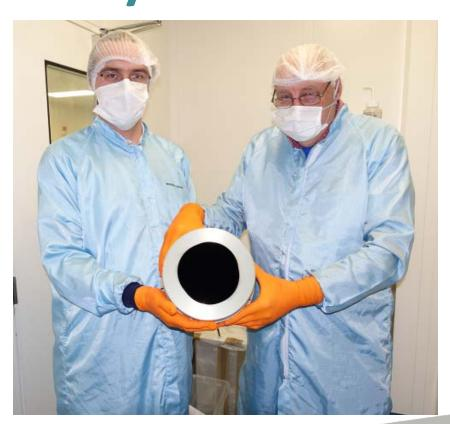
Coated base and wall to complete flight like cavity
