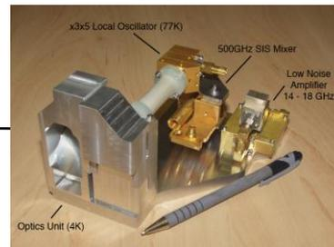
RAL ultra-compact 500 GHz SIS radiometer subsystem
