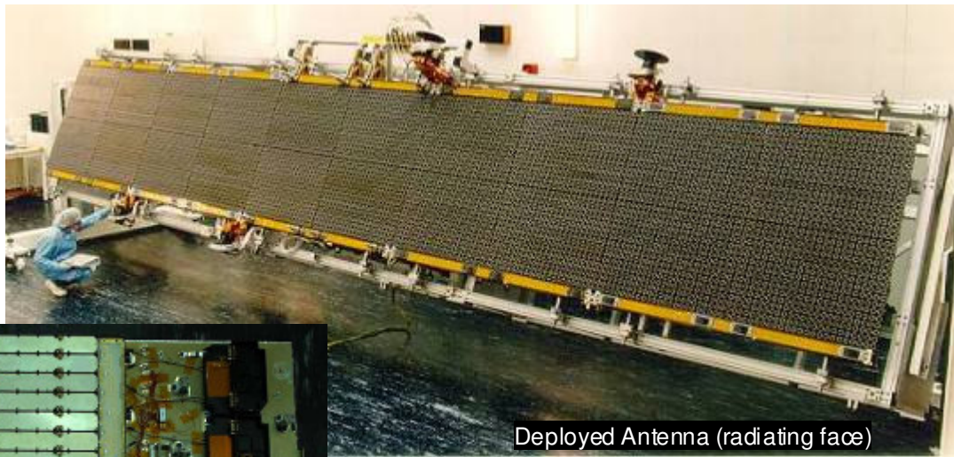
Floating-floor deployment testing
