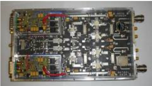
GaN Transmit Unit
