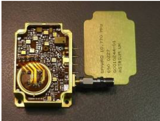
Ovenised Resonant Oscillator (Astrium SpHARO)
