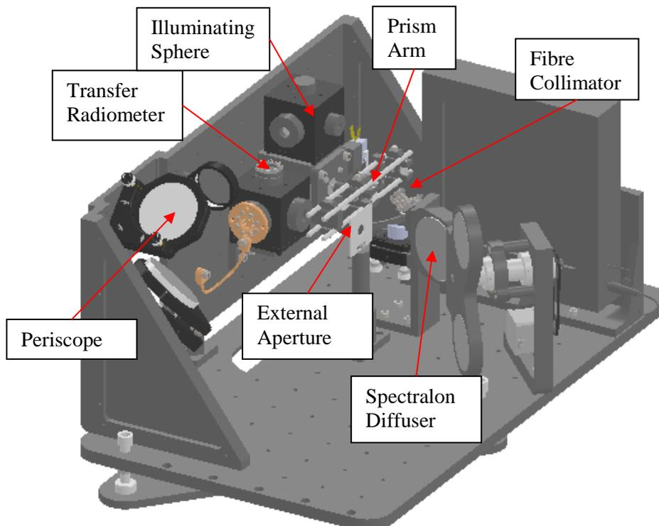
**Figure 3 CAD model of prototype calibration system. CSAR is viewable in one of the positions of the prism arm behind the back plate of the system, while the EI would view the diffuser at a 45 degree angle.**
