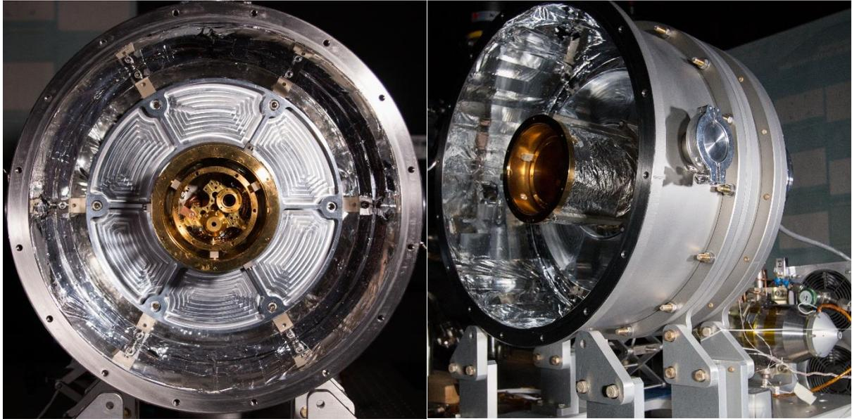
**Figure 1 (Left) CSAR instrument mounted on cold tip of HPSC inside cryostat. (Right) Side view showing integration of HPSC into cryostat.**
