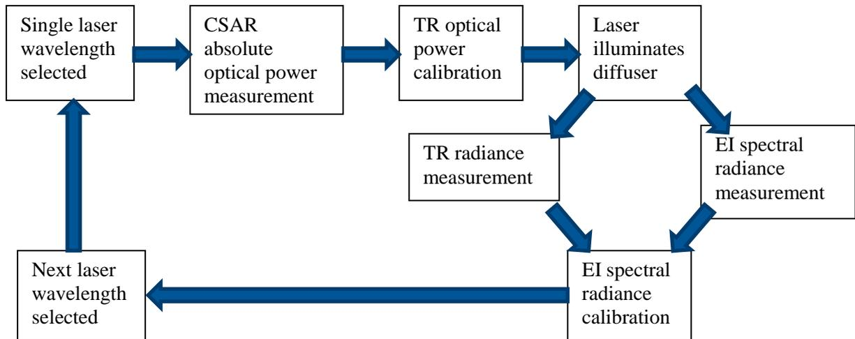
**Figure 2 Schematic showing calibration chain of TRUTHS calibration system.**
