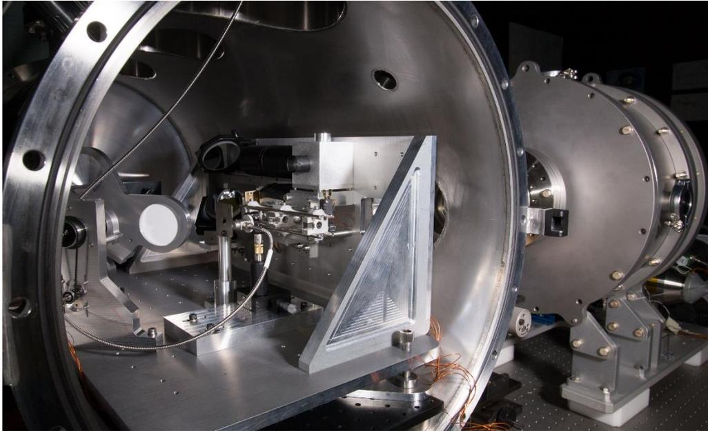
**Figure 4 Photograph of calibration system prototype installed in vacuum tank and coupled to CSAR cryostat and HPSC.**
