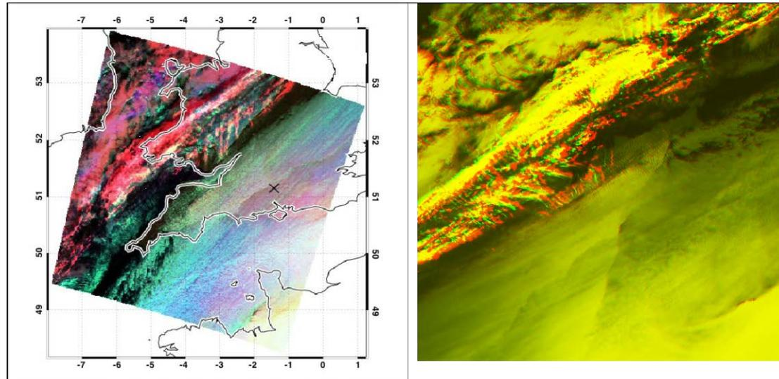
ATSR2 Stereo CTH retrieval at  $1.6\mu\text{m}$  (left) and  $11\mu\text{m}$  (right)
