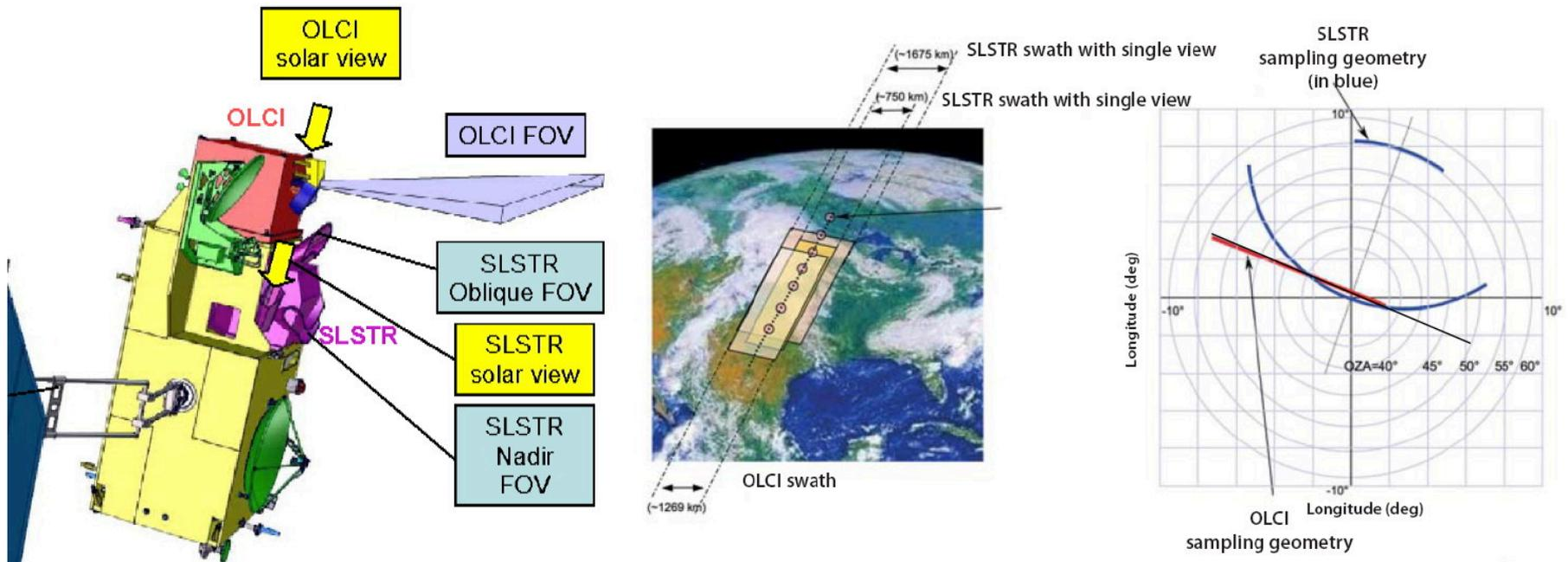
SLSTR 750km overlap could provide stereo (750m) winds from polar
