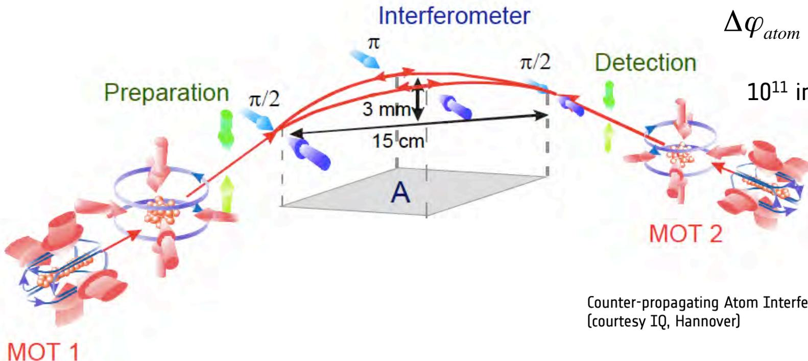
Counter-propagating Atom Interferometers scheme
