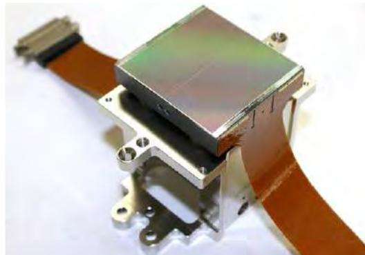
e.g. p-channel CCD evaluation, for improved radiation tolerance
