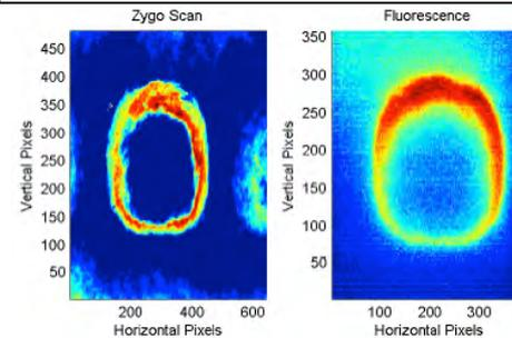
3D strain mapping in composite materials
