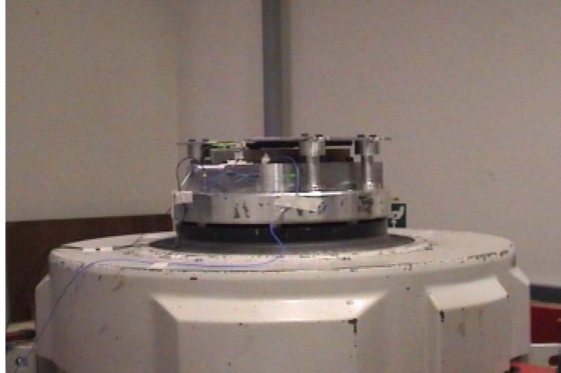
Vibration testing of the qualification pair of LISA Pathfinder fibre injectors at Selex ES
