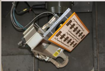
Airborne Demonstrator Back End Electronics X-band / S-band Front End Electronics X+S-band Antenna/Gimbal Assembly
