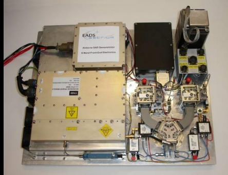
Airborne Demonstrator Central Electronics 215MHz configuration X band wideband Front End
