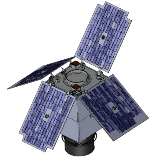
Deployed imager accommodated on the SSTL-42 platform
