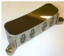
Selective laser melting Mass: 127.7 g Material: Ti6Al4V 1 st eigen freq ~2100 Hz NiP coating
