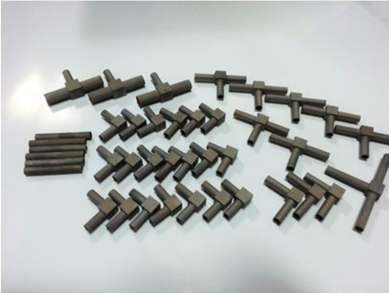
Sample components (Produced from the same drawings as conventionally machine components).
