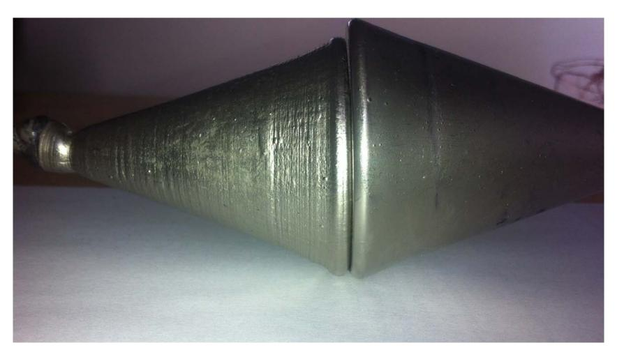
Linear shrinkage in line with expected shrinkage from consolidation of tap density powder
