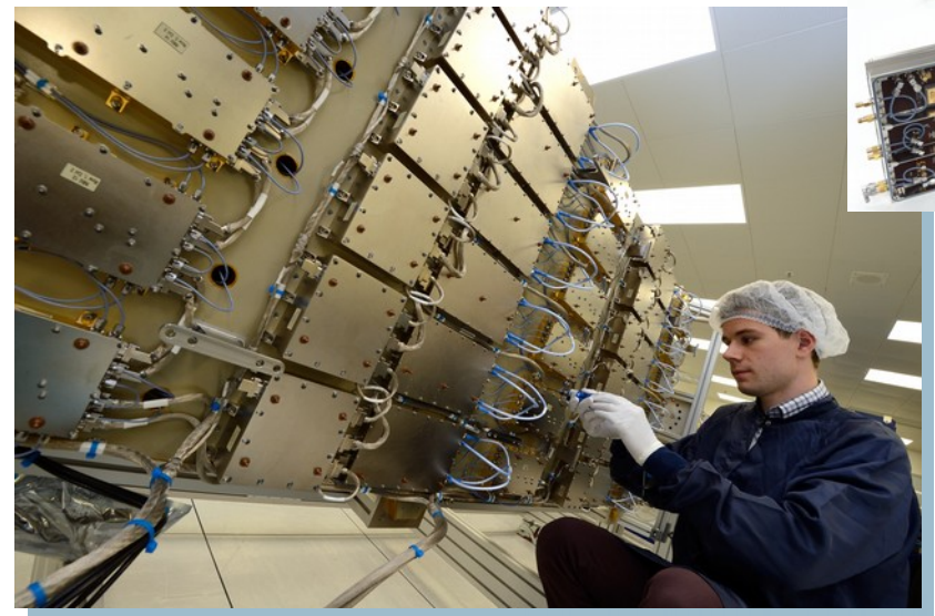
NovaSAR-S FM Antenna integration
