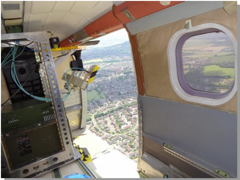
Sensor operations with no radome on Twin Otter
