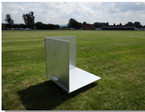
Calibration target for AirSAR flight trials
