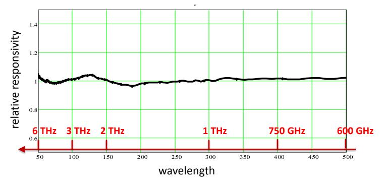
• no spectral absorption features due to the thin PVDF foil
