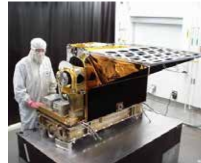
AIRS Instrument on AQUA
