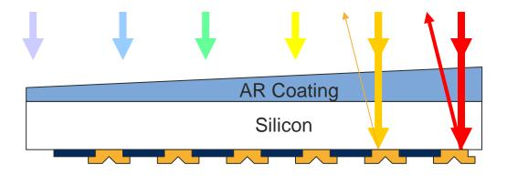
But note that at longer wavelengths the silicon becomes transparent and so reflections are seen from the front surface.
