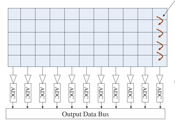
Charge is transferred within the array in a similar manner to a CCD
