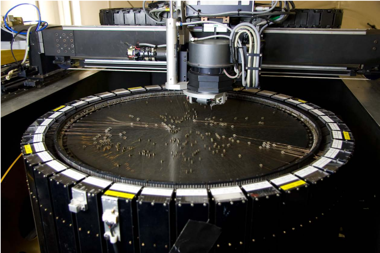
The 2df multi-object robotic optical fibre positioner
