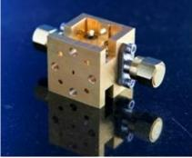
SHIRM 360 GHz image separator mixer using Schottky diode technology
