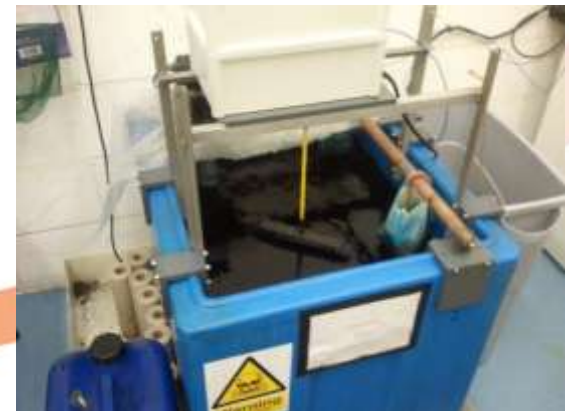
Electroforming of diplexers
