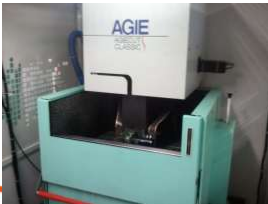
Wire erosion of mandrel blank
