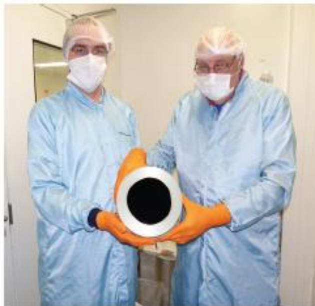
Figure 4: Breadboard blackbody cavity with carbon nanotube Vantablack © coating developed by Surrey NanoSystems (SNS) under an NSTP-2 project
