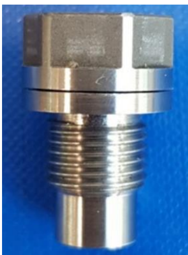
Figure 1: Left: phase-change cell. Right: phase-change cell immersed in aluminium block, also showing thermometer.
