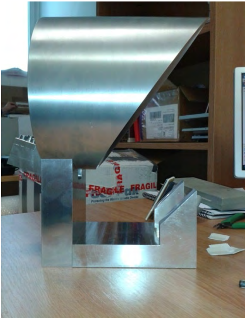
Full setup with Electronically Tunable LC Reflectarray Subreflector
