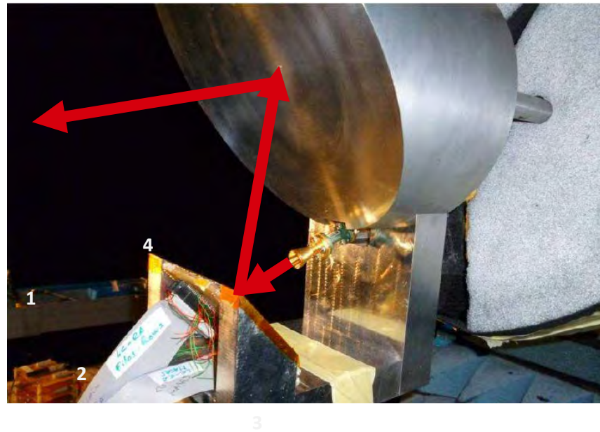
Full setup with Electronically Tunable LC Reflectarray Subreflector
