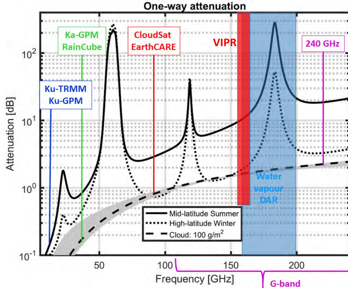
Absorption band freq  $\rightarrow$  water vapour profiling in the 183 band
