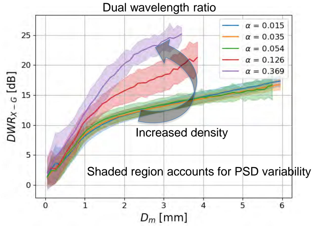
Larger DWRs  $\rightarrow$  G band observations have potential for quantitative retrievals of smaller size crystals compared to those achievable by using longer wavelengths.
