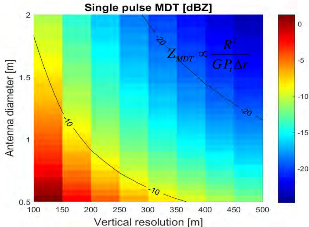
Thus better sensitivity than CloudSat (EarthCARE) which have a single pulse MDT of  $-16.5$  dBZ ( $-21.5$  dBZ)
