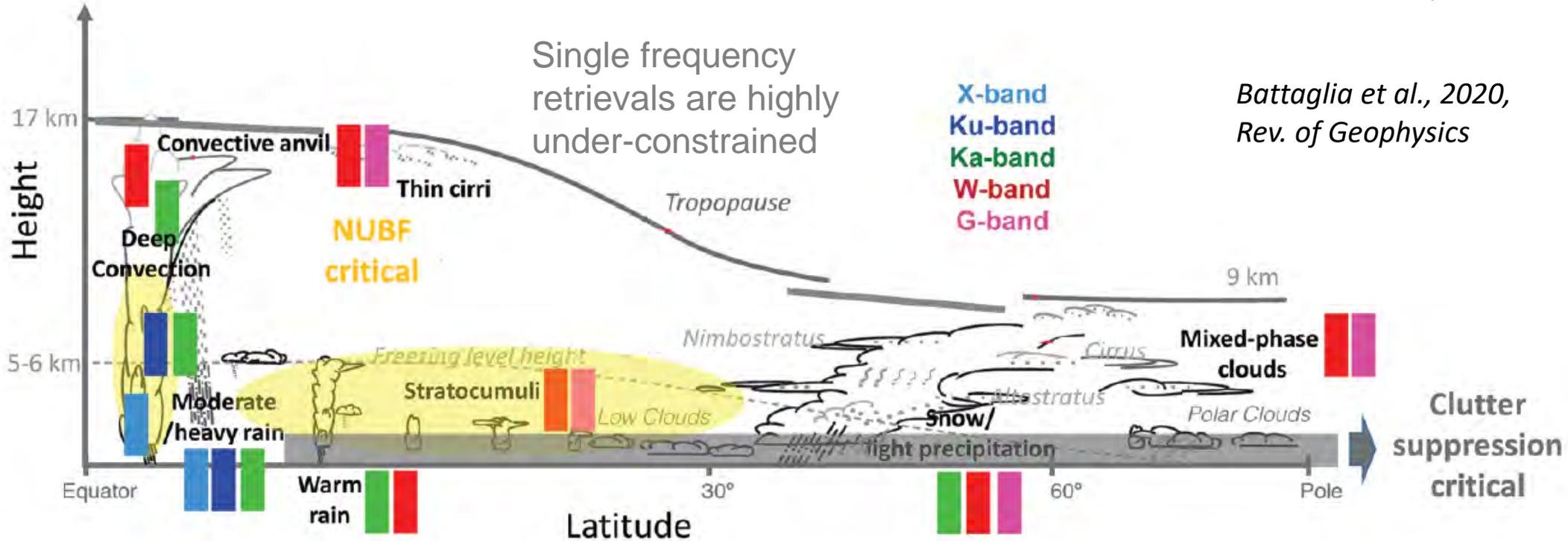
**Solution:** combination of multi-frequency (Doppler) radars with frequencies ranging from 10 to above 200 GHz allows characterizing from heavy precipitation particles to small-size ice crystals. Inclusion of G-band (1.5 mm) highly beneficial in three areas: **boundary layer clouds, cirrus and mid-level ice clouds and precipitating snow.**
