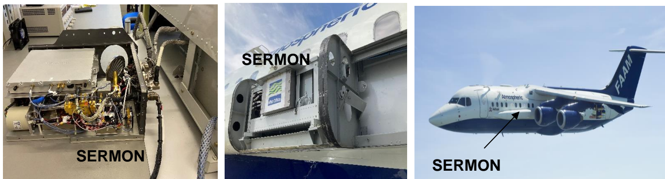
The HYMS demonstrator instrument (SERMON) ready for airborne deployment is shown on the left. It is mounted on the FAAM aircraft (middle) for atmospheric sounding proof-of-concept. The FAAM BAE 146 aircraft used for airborne deployment is shown on the right. (Image credit: RAL Space, STFC)
