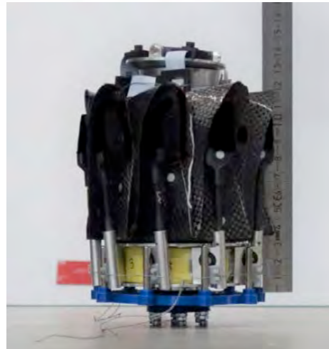
Centre-fed REVOLVE "origami-folded" reflector, 0.5m, Ka-band (credit: LSS GmbH).
