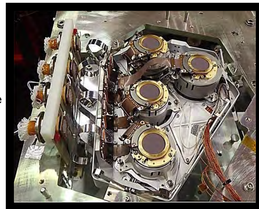
Band 1,2,3,4 detectors mounted into the flight cryostat at Airbus Toulouse
