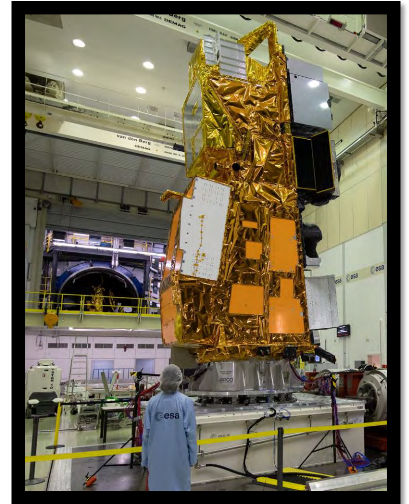
MetOp-SG on the Shaker at Airbus
