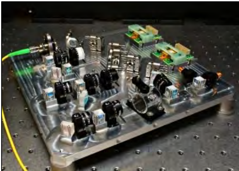
Tunafish: Fibre-coupled rubidium- and offset-locked laser system.
