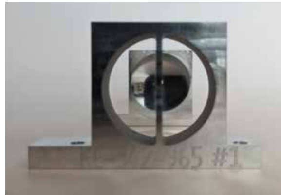
Front end telescope 25 mm aperture
