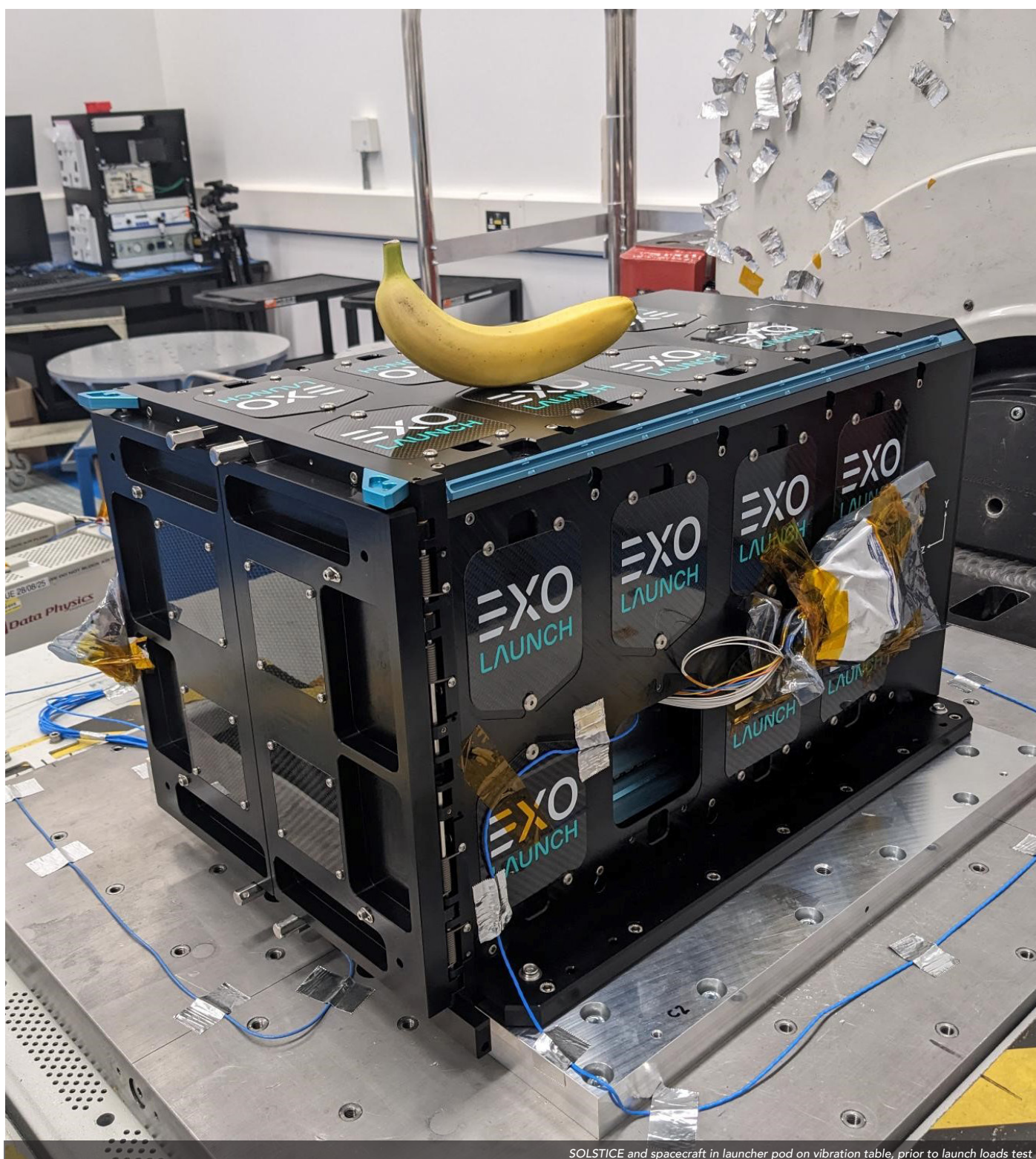
SOLSTICE and spacecraft in launcher pod on vibration table, prior to launch loads test
