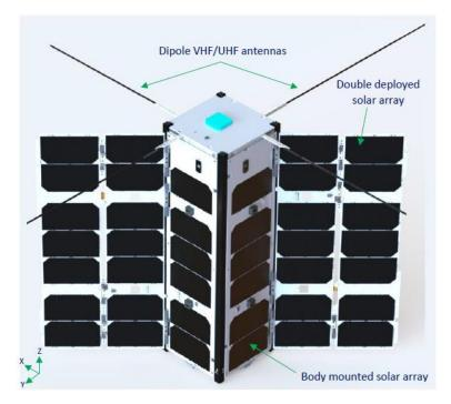
Figure 2.1 - Deployed CSL 3U Platform ©Clyde Space Ltd
