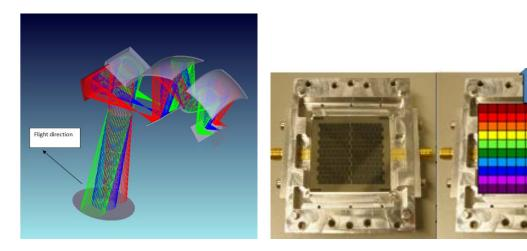
Figure 1. Left: Wide FOV fore-optics coupled to detector array via re-imaging optic and reflective cold stop. Right: Indication of multispectral/hyperspectral imaging configuration. Flight direction is indicated by the arrow. Across-track direction is spatial domain, along-track direction is spectral domain.
