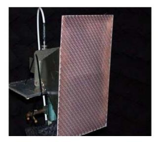
Electromagnetic Band Gap (EBG) polarisation transformer
