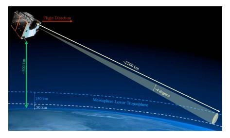
Illustration of the LOCUS limb-sounding radiometer in operation.
