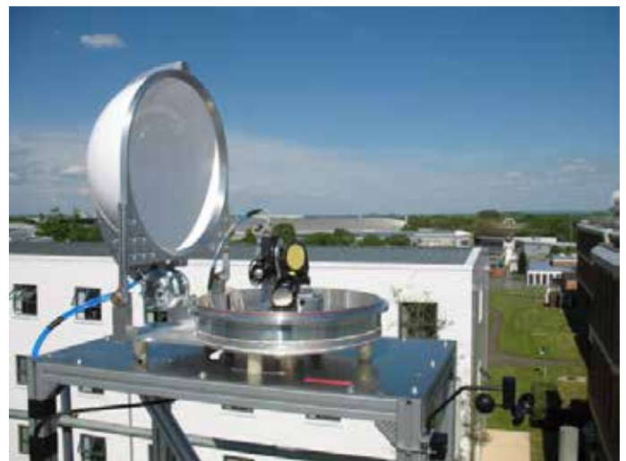
Rooftop mounted passive solar tracking system developed for ground based CO 2 measurement by LHR
