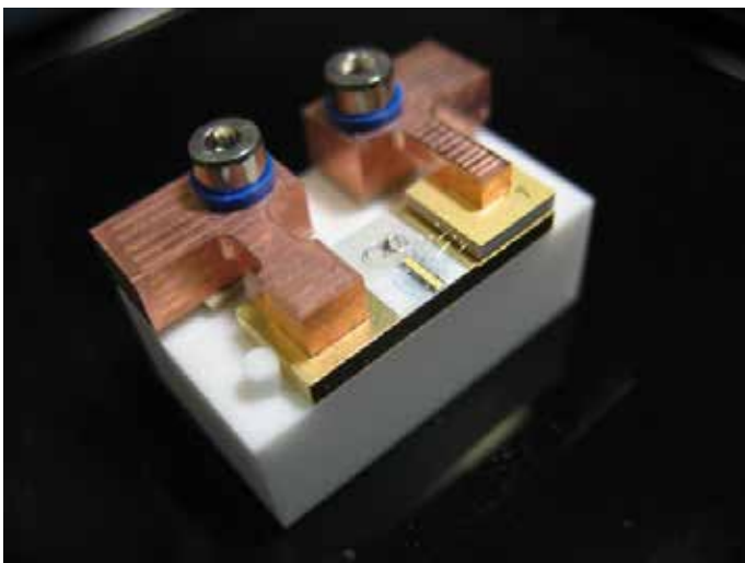
Quantum cascade laser local oscillator at the core of the LHR. The laser dimension are 0.5x0.3x3 mm 3
